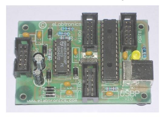
The compact USB PORT Module from eLabtronics can be used as a PIC programmer and a controller. It programs user PIC projects using the eLabtronics industry strength CoreChart graphical assembler or PIC machine code ( hex ) files. You can find a full version 30day FREE trial copy of CoreChart at www.elabtronics.com
