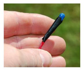
Use insulation tape (when working with relatively low temps) or good quality heatshrink (high temp sensing) to insulate the connections.
