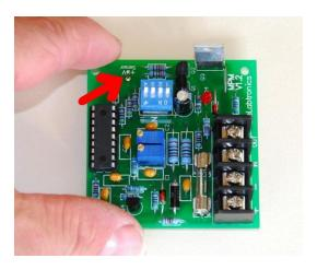
To automatically trigger the Pulser on the basis of temperature or light intensity, use is made of a regulated 5V supply sourced from the module. This is available on the pin shown here.
